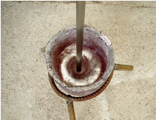
Fig. 2. Mixing the carbon fiber with the aluminum matrix by making a vortex flow.
