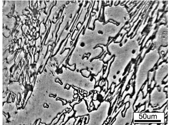
Fig. 1. The microstructure of the as-cast high-chromium cast iron.
