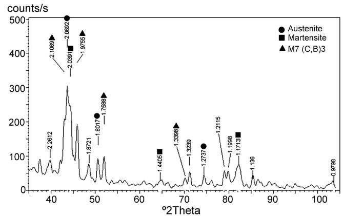
Fig. 2. The XRD pattern of the as-cast high-chromium cast iron.
