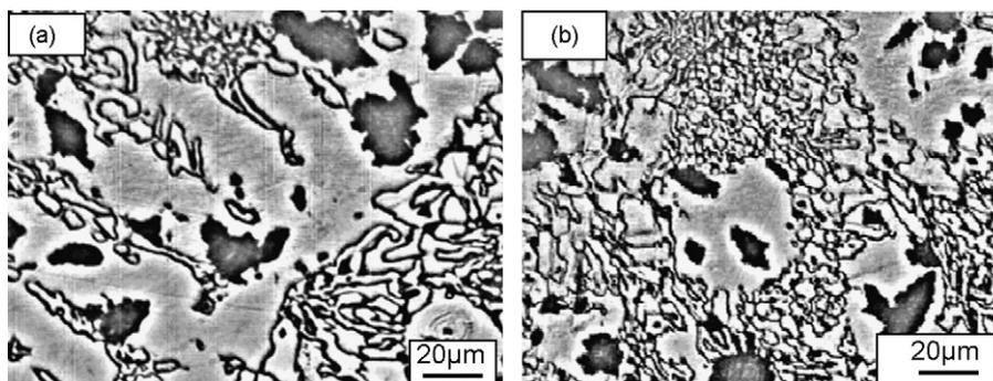
Fig. 3. The microstructure of the high-chromium cast iron: (a) air cooling after sub-critical treatment at 550 °C and (b) cryogenic treatment after sub-critical treatment at 550 °C.
