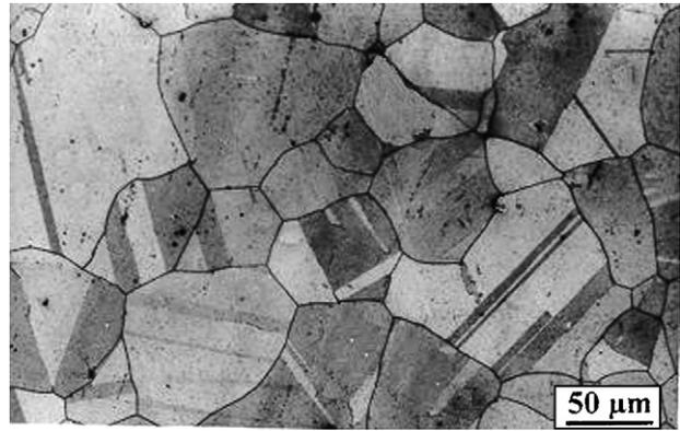
Fig. 1. Optical micrograph of the Fe–Ni–Cr–Al alloy in solution treated condition.
