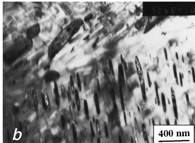
Fig. 2. Transmission electron micrographs revealing morphology of NiAl precipitates in the Fe–Ni–Cr–Al alloy in (a) peak (973 K/5 h) and (b) overaged condition (973 K/50 h).
