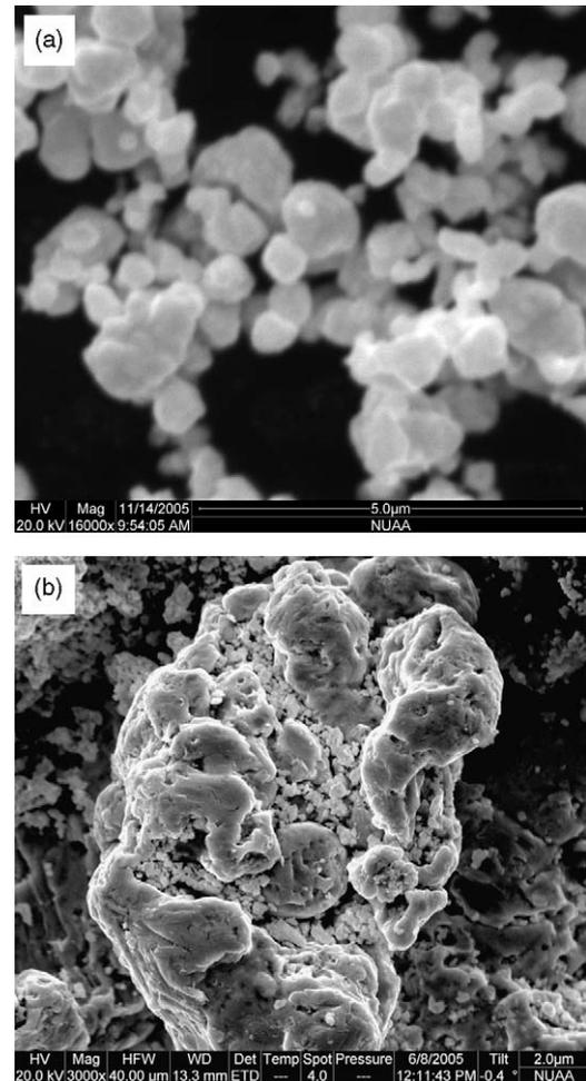
Fig. 1. SEM images showing characteristic morphologies of the WC–Co composite powder (a) and the mixed powder system (b).
