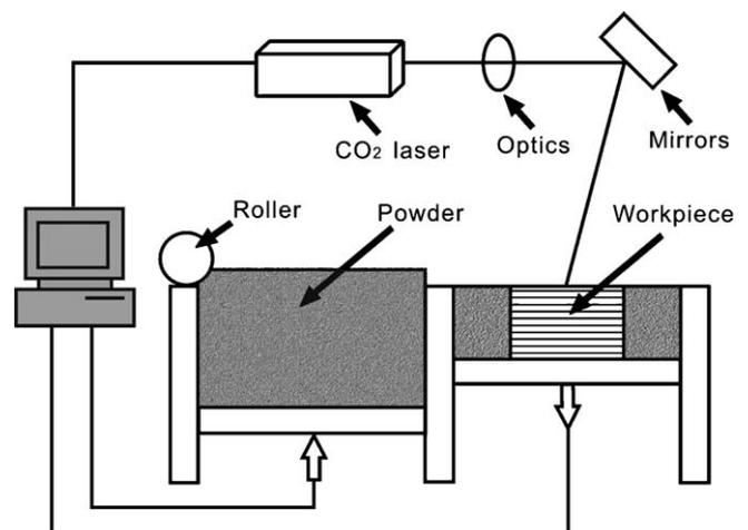
Fig. 2. Schematic diagram of the direct laser sintering apparatus.
