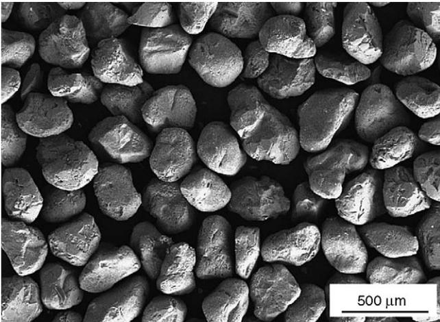
Fig. 1. Micrograph of sandblasting particles.
