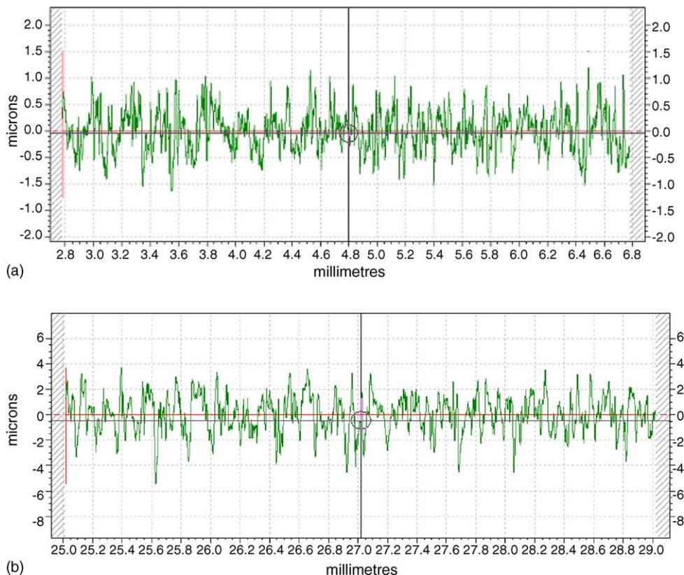
Fig. 2. Surface roughness of: (a) the untreated titanium and (b) sandblasted titanium.
