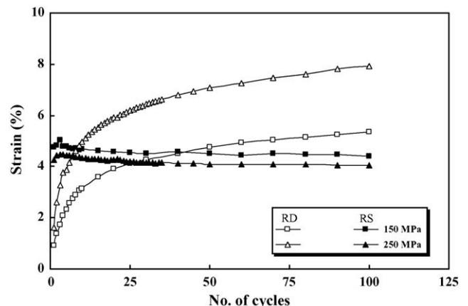
Fig. 3. Strain (RS and RD) vs. number of cycles plot of a Ni–Ti–Cu SMA wire actuator during TMC.
