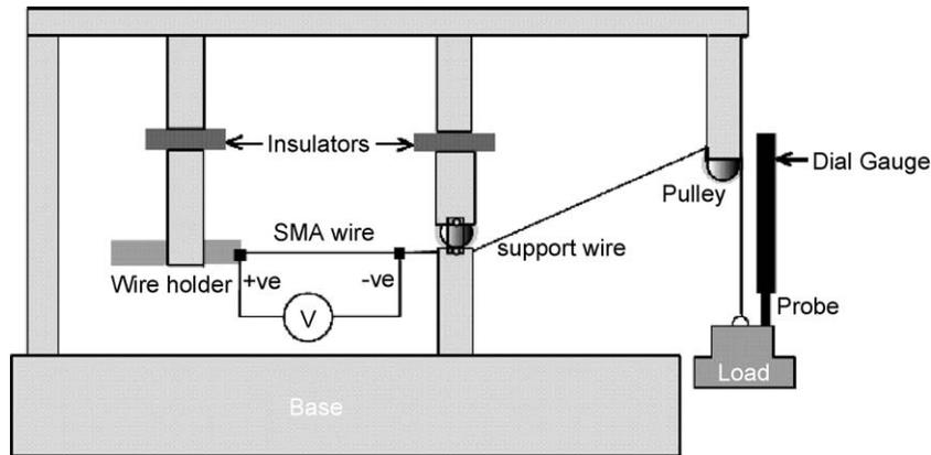
Fig. 1. Schematic of the thermo-mechanical cycling set-up.
