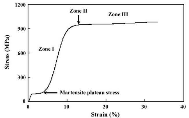
Fig. 2. Stress–strain diagram of Ni–Ti–5.5 at.% Cu SMA wire tested in martensite phase at 23 °C.
