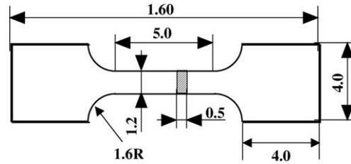
Fig. 1. Dimensions of miniaturized tensile specimen.
