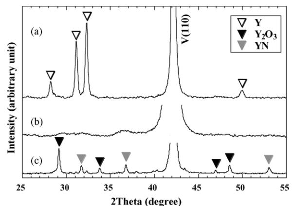
Fig. 2. X-ray diffraction patterns taken from (a) mixed powder of the starting materials, (b) MA processed powder and (c) as-HIPed specimen of V–1.7Y.
