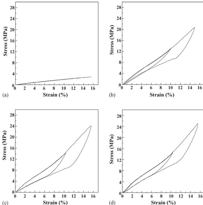
Fig. 2. The nominal stress–strain curves generated by single TiNi ring in different pre-strain states, without sliding blocks (a) and the pre-strains of the ring are 0 mm (b), 4.17% (c) and 8.33% (d), respectively.
