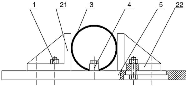
Fig. 1. Scheme of damping device: (1) bolts for the fixation and adjustment of sliding blocks, (21 and 22) sliding blocks, (3) shape memory alloy rings, (4) fastening bolt of the rings and (5) foundation plate.
