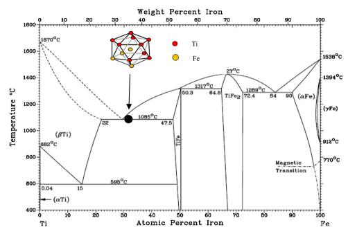
Fig. 1. Ti-Fe binary phase diagram and Ti<sub>9</sub>Fe<sub>4</sub> cluster structure.
