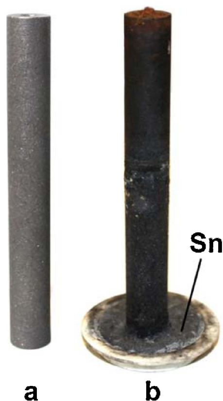
Fig. 2. Photographs of a graphite rod (a) before and (b) after being used as the cathode during the electrolysis of LiCl-30 wt% SnCl 2 . The molten salt electrolysis was conducted at 770 °C for 2 h at the constant current of 33 A, corresponding to an initial cathode current density of about 1 A cm -2 . Details of the set-up used can be found in [11].
