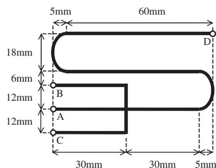
Fig. 1. A schematic of the cross-mixer channel (rectangular channel,  $500 \mu\text{m} \times 500 \mu\text{m}$ ). A is the inlet of Dimethicone, B is the inlet of the aqueous solution mixture of  $\text{CH}_3\text{COONa}$ , KI, and  $\text{KIO}_3$ , C is the inlet of the HCl aqueous solution, D is the outlet.
