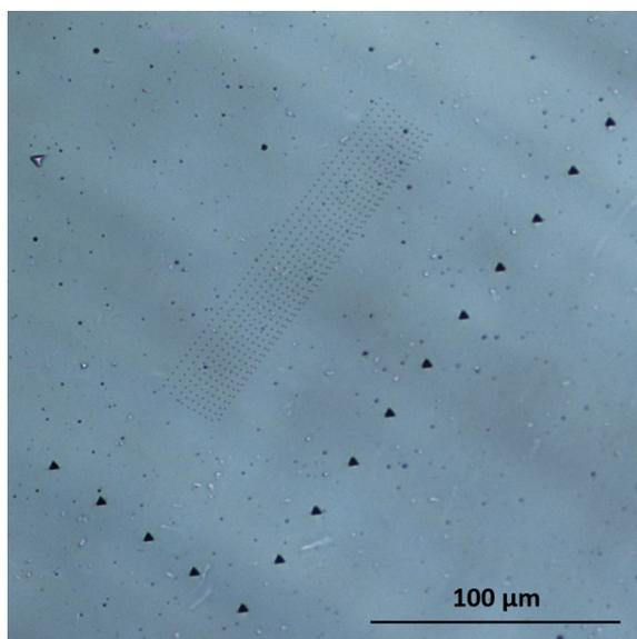
**Fig. 1.** Optical microscopy image showing the area of interest (in the center of the image) constituted of an array of nano-indentations at the sample surface, surrounded by micro-indentations forming an L-shaped pattern.
