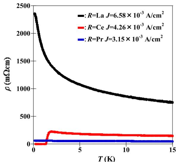
Fig. 2. (Color online)  $\rho$ - $T$  characteristics of ROBiS<sub>2</sub> poly-crystalline samples at 0.13–15 K using ADR option.
