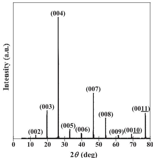
Fig. 3. XRD pattern of well-developed plane of CeOBiS<sub>2</sub> single crystal.
