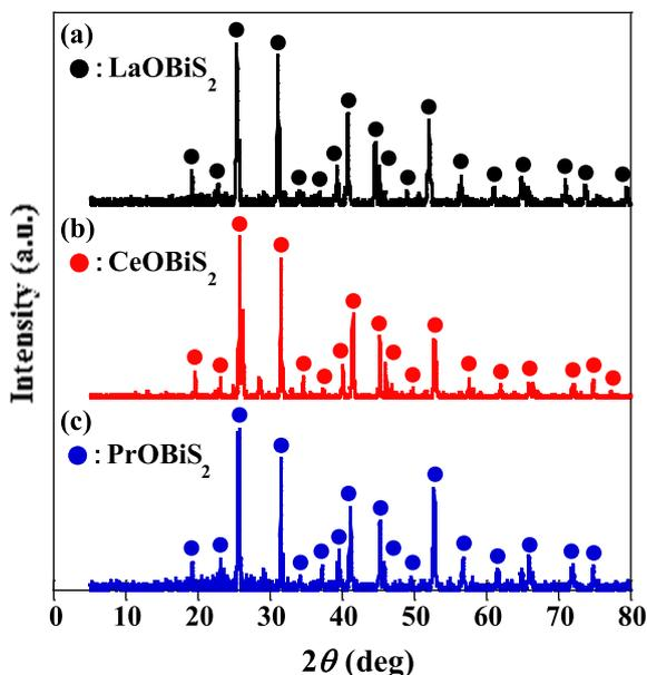
Fig. 1. (Color online) XRD pattern of ROBiS<sub>2</sub> poly-crystalline samples where (a)  $R=\text{La}$ , (b)  $R=\text{Ce}$  and (c)  $R=\text{Pr}$ .
