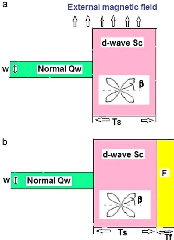
**Fig. 1.** (Color online) Schematic representation of the system under study: (a) a normal quantum wire–d-wave superconductor junction in an external magnetic field which is a “Zeeman-split” superconductor layout; (b) a normal quantum wire/d-wave superconductor/ferromagnetic metal, where an exchange field is induced by a ferromagnetic layer which is in contact with superconductor and induced the ferromagnetism via the proximity effect.
