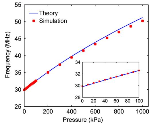
Fig. 2. (Color online) Resonance frequency versus applied pressure from 0 to 1000 kPa using finite element simulation and theoretical expressions. The inset shows the linear relationship when pressure ranges from 0 to 100 kPa. Good agreement is obtained using the two methods.
