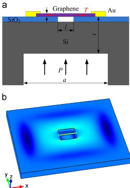
Fig. 1. (Color online) (a) The schematic of the pressure sensor chip under the measured pressure. (b) X component of stress tensor calculated using the finite element simulation; the resonant beam shows tensile stress under pressure.
