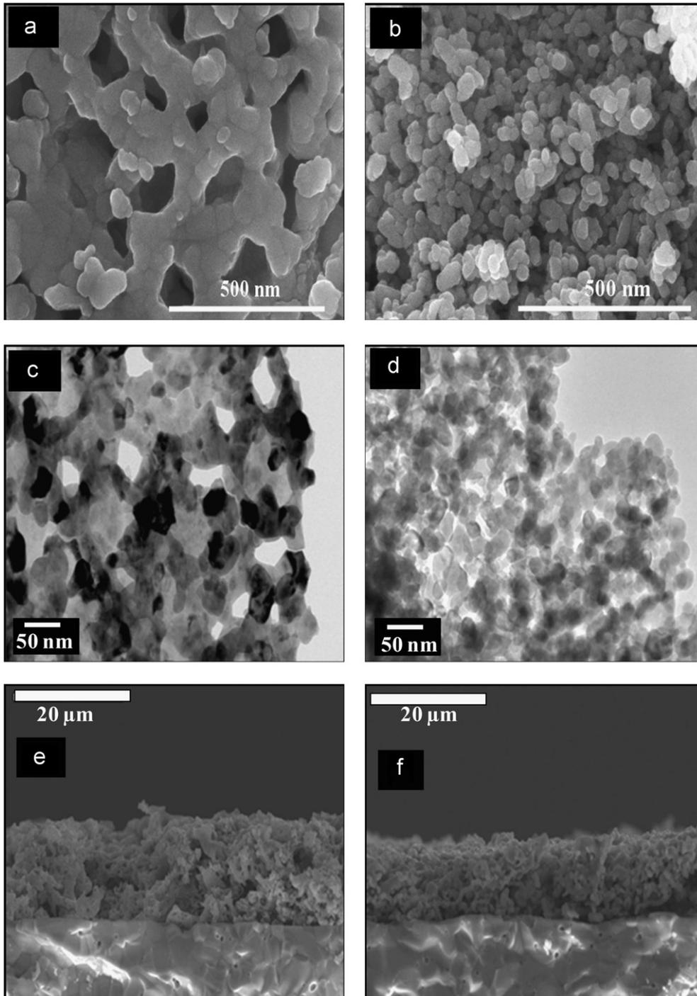
**Fig. 2.** SEM (a and d) and TEM (b and e) images of the powders synthesized at 700 °C for PSF (a and b) and PSFCu (d and e). Cross-section view of SDC-PSF (c) and SDC-PSFCu (f) interface.
