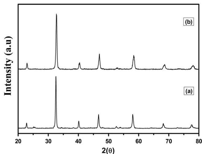
Fig. 1. The XRD patterns of PSF (a) and PSFCu and (b) synthesized at 700 °C.
