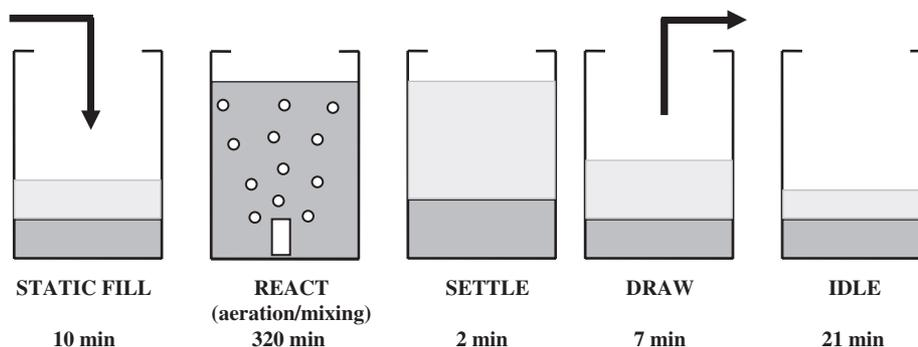
Fig. 1. Scheme of the sequencing batch reactor (SBR) cycle.
