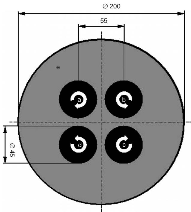
Fig. 1. A schematic illustration of the 4RM. (a)–(d) rolls, (e) sample chamber. Dimensions in mm.
