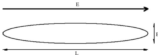
Fig. 2. A schematic illustration of the elliptic/elongated drop.  $L$  is the length and  $B$  the diameter of the drop.  $E$  shows the direction of the elongation field.
