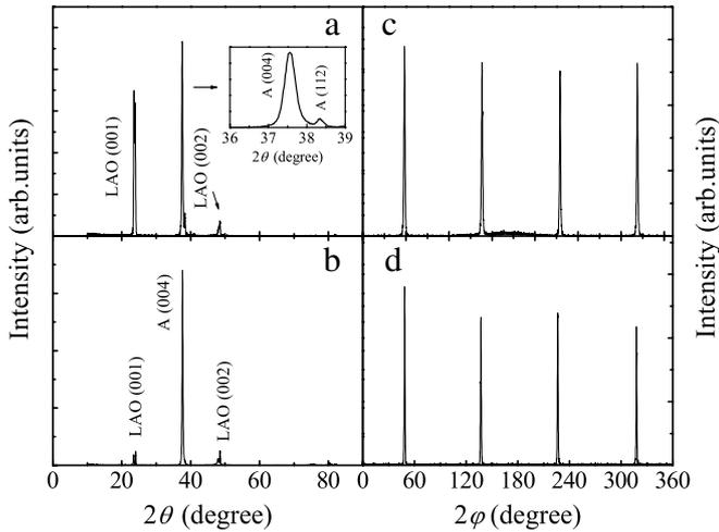
**Fig. 1.** XRD  $2\theta$  spectra for (a) Sample A and (b) Sample B, and XRD  $\varphi$ -scan spectra for (c) Sample A and (d) Sample B.
