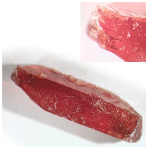
Fig. 1. Single crystal of guanidinium \text{Co}^{\text{II}} sulphate hexahydrates (longest dimension 1.4 cm). Small detail: the crystals easily undergo plastic deformation and are therefore (unfortunately) unsuited for cutting or polishing.
