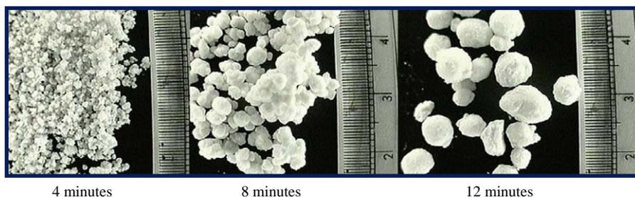
Fig. 1. Granulation test in a planetary mixer: Influence of granulation time on product; 18% water (wt solids). Water addition to lactose (96 wt%) PVP (4 wt%).
