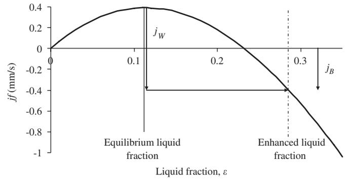
Fig. 1.  $j_f$  versus  $\epsilon$  for a pneumatic foam showing the graphical calculation of equilibrium liquid fraction, enhanced liquid fraction due to washwater rate  $j_w$  and the definition of bias rate,  $j_B$  (after Stevenson, 2007b).
