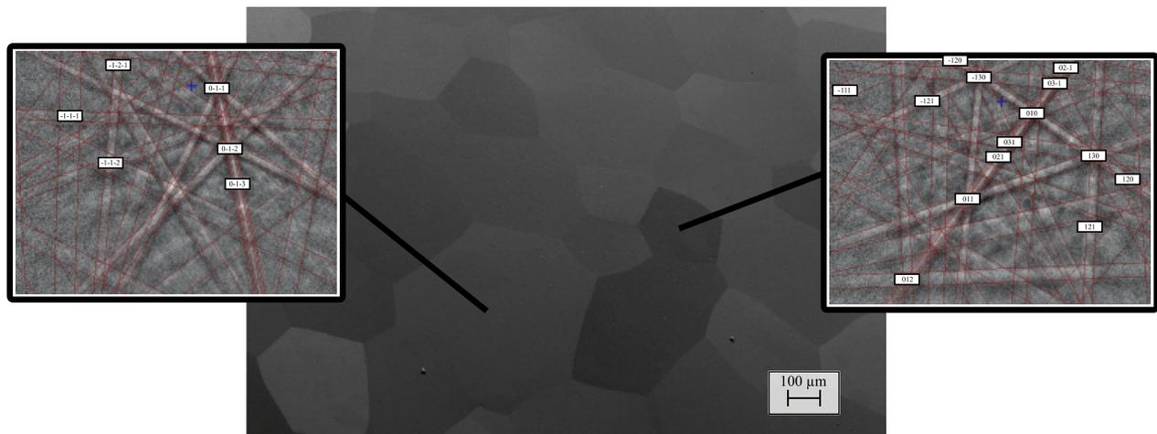
Fig. 1. Single phase ( $\eta$ -AlFe) SEM-micrograph (BSE) of the annealed S2-I (71.67 at.% Al) sample after heat capacity measurements together with two indexed EBSD patterns using the orthorhombic structure model by Burkhardt et al. [5].
