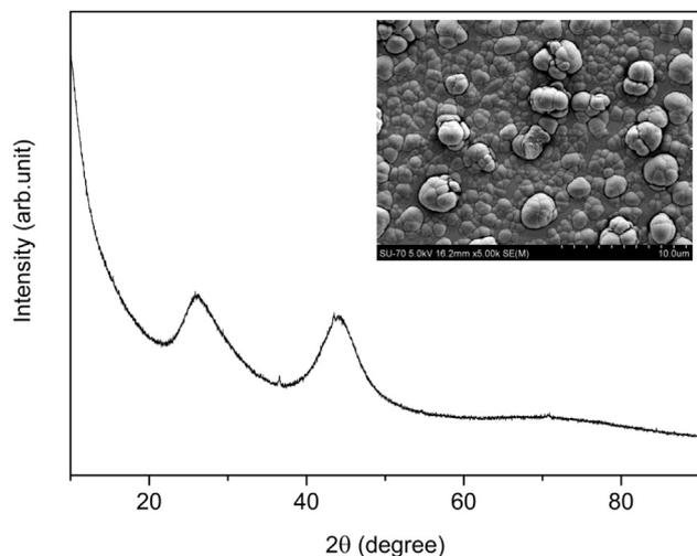
Fig. 1. XRD pattern and surface morphology of as-deposited Zn–Sb based thin film.
