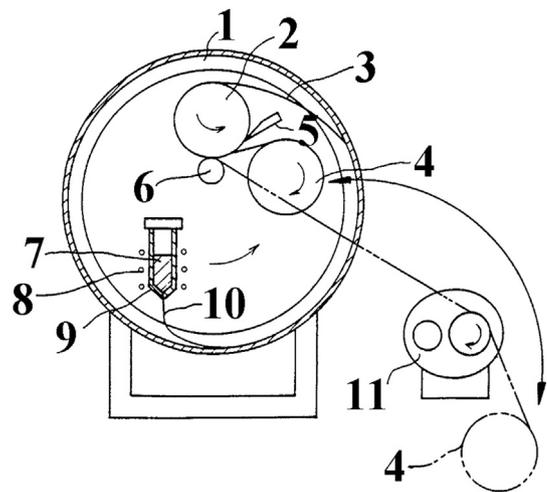
**Fig. 2.** Schematic illustration of the in-rotating-water spinning apparatus combined with a winder. 1. Rotating drum; 2. First magnet roller; 3. Wire specimen; 4. Second magnet roller; 5. Scraper; 6. Nip roller; 7. Molten alloy; 8. High frequency coil; 9. Melting crucible; 10. Ejected alloy; 11. Winder [26].
