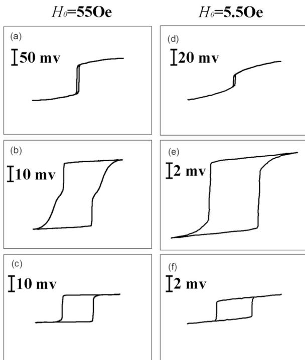
**Fig. 1.** BH loops of  $\text{Fe}_{75}\text{B}_{15}\text{Si}_{10}$  (a, b, c) and  $\text{Co}_{72.5}\text{B}_{15}\text{Si}_{12.5}$  (d, e, f) glassy wires with  $d_0 = 125 \mu\text{m}$ . (a) and (d): as quenched; (b) and (e):  $R = 20\%$ ; (c) and (f):  $R = 80\%$  [25].
