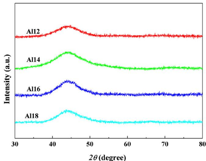
Fig. 2. XRD patterns of as-cast  $Zr_{56}Co_{44-x}Al_x$  ( $x = 12, 14, 16$  and  $18$ , respectively) alloys showing typical broad diffraction maxima without any detectable crystalline peaks, indicating fully amorphous nature.
