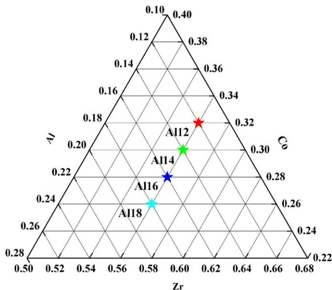
Fig. 1. Schematic phase diagram displaying the investigated  $Zr_{56}Co_{44-x}Al_x$  ( $x = 12, 14, 16$  and  $18$ , labeled as Al<sub>12</sub>, Al<sub>14</sub>, Al<sub>16</sub> and Al<sub>18</sub>, respectively) glassy alloys.
