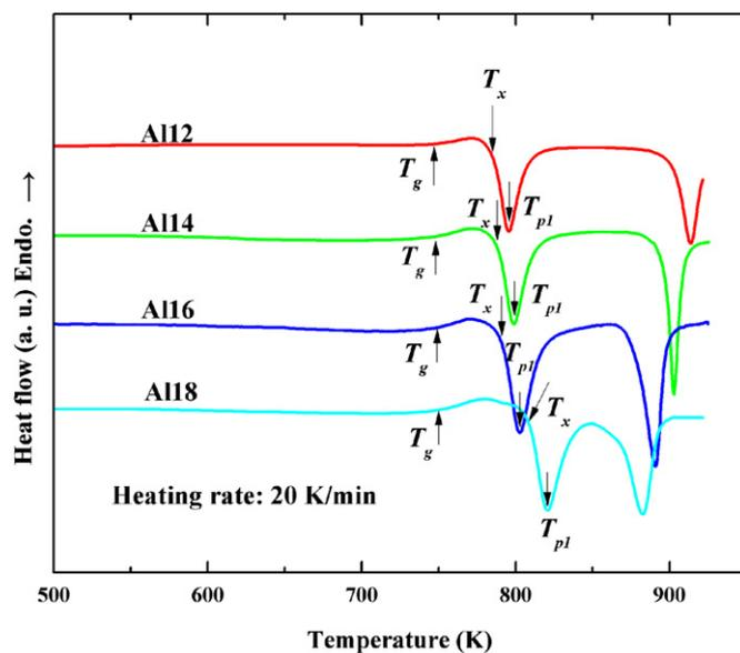
Fig. 3. DSC curves of  $Zr_{56}Co_{44-x}Al_x$  ( $x = 12, 14, 16$  and  $18$ , respectively) glassy alloys at a heating rate of 20 K/min. The glass transition temperature ( $T_g$ ), the onset temperature of crystallization ( $T_x$ ), and the temperature of the first crystallization peak ( $T_{p1}$ ) are marked with arrows.
