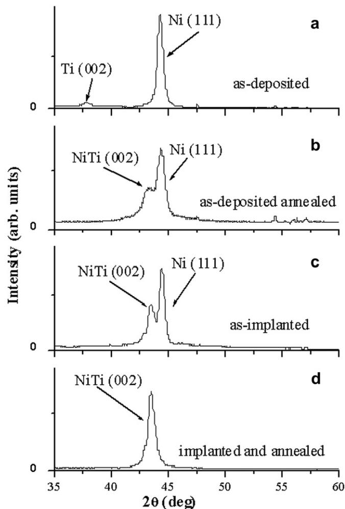
Fig. 1. XRD spectra of the (Ni/Ti)<sub>x</sub>/Si multilayer structure: (a) as-deposited, (b) annealed at 400 °C, (c) as-implanted with Ar<sup>+</sup> ions to  $6 \times 10^{16}$  ions cm<sup>-2</sup>, and (d) Ar-ion implanted and annealed samples.
