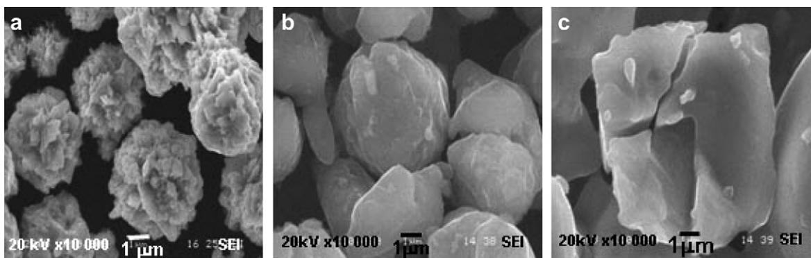
Fig. 1. SEM micrographs of the elemental powders: (a) Ni, (b) Al and (c) Ti.
