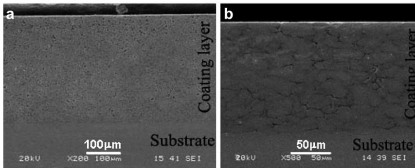
Fig. 2. SEM images of coated samples: (a) NiAl and (b) TiAl.
