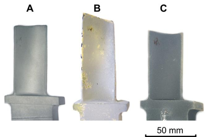
Fig. 1. The overview of TiAl turbine blades: (A) after aluminizing, (B) after 1000 h oxidation test (without aluminizing) (C) after aluminizing and 1000 h oxidation test.
