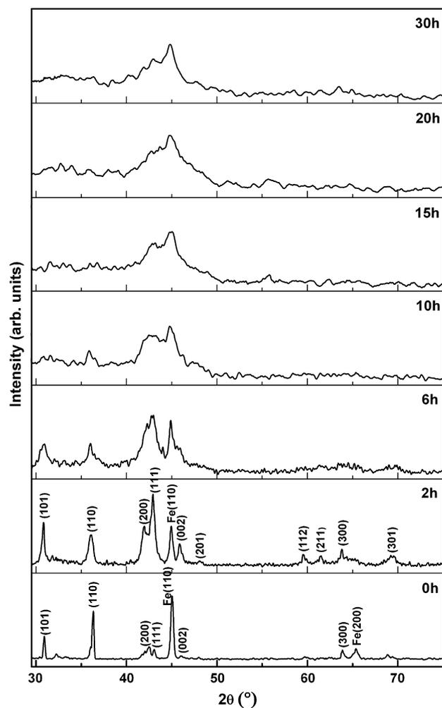
Fig. 1. X-ray diffraction patterns of as-milled  $\text{SmCo}_5/\alpha$ -Fe nanocomposite powders for various milling times. The Miller indices of the main diffraction peaks are indicated in the figure.
