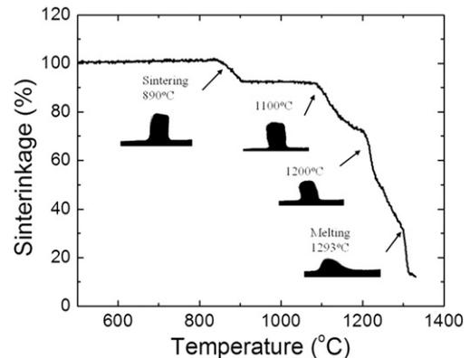
Fig. 2. Variation in shrinkage for MCAS glass powder compact. Images on its morphological change are also inserted inside this plot.
