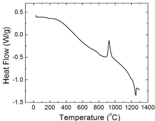
Fig. 1. DTA scans of MCAS glass oxide powder used as a sintering additive of AlN in this study.
