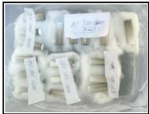
Fig. 2. Green compact of the specimen.
