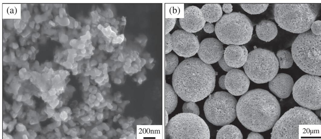
**Fig. 1.** Typical morphologies of (a) the as-synthesized nanoscale WC–12Co composite powder and (b) the spray-dried composite powder particles.
