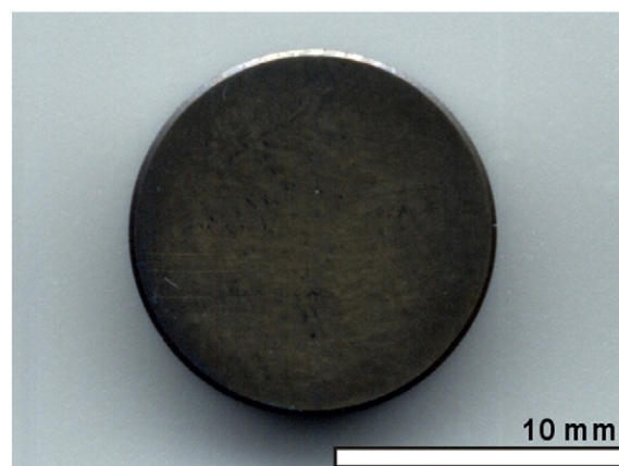
Fig. 2. DTi_3(Si,Ge)C_2 specimen after lapping and polishing.
