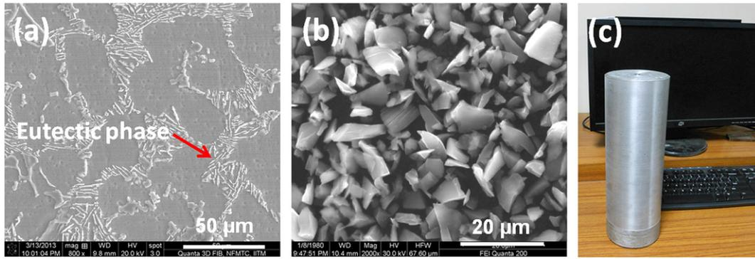
Fig. 1. (a) Microstructure of the etched  $Al_m$  (Al-12%Si alloy), (b) HRSEM image of the raw SiC particles and (c) photograph of the casted  $Al_m$ -30%SiC<sub>p</sub> ingot.
