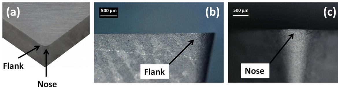
Fig. 2. Views of the tool cutting edge. (a) Isometric view, (b) flank face and (c) nose.
