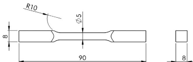
Fig. 1. Sample dimensions (in mm).
