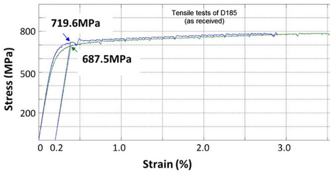
Fig. 2. Stress–strain curves for D185 alloy at 25 °C.
