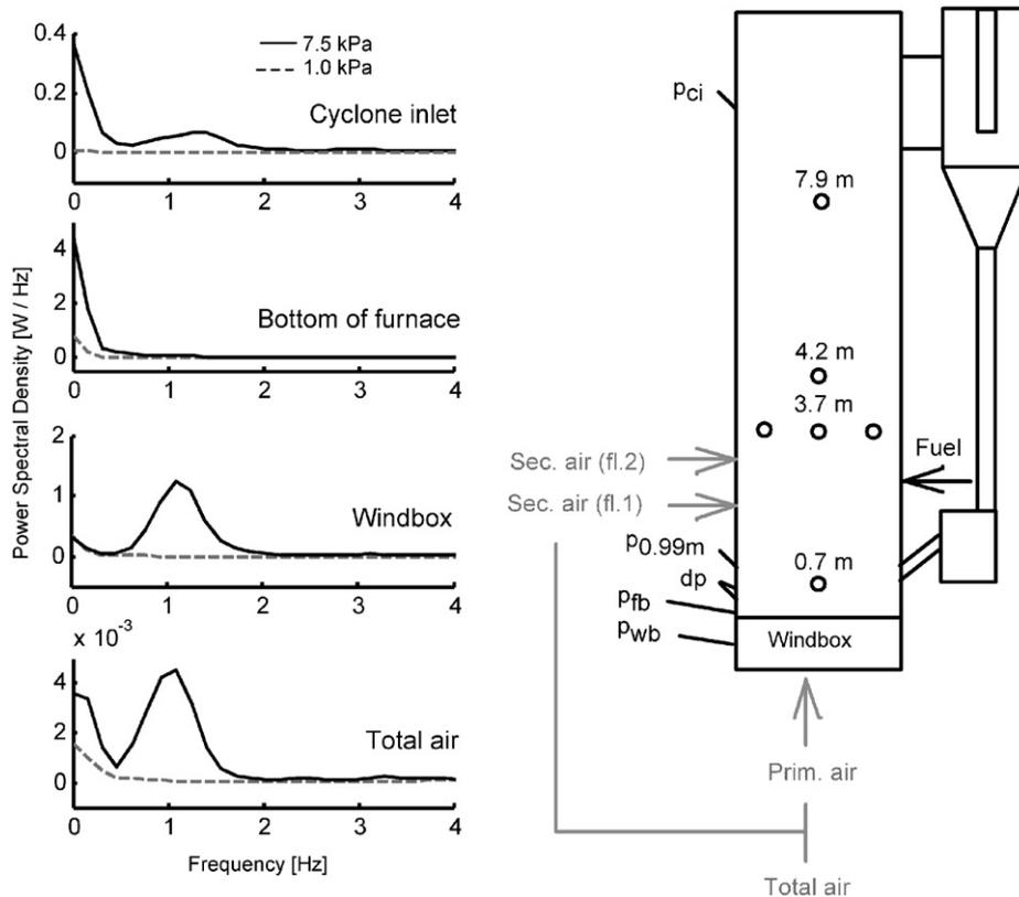
Fig. 1. Examples of power spectral densities at various positions in the furnace in the reference case and the case without a bottom bed.
