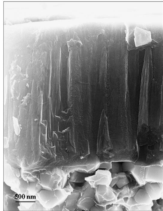
Fig. 1. SEM fracture cross-sectional image of Ti-Al-N single layer.
