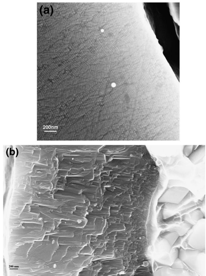
Fig. 2. SEM cross-section images of TiN/TiAlN nano-multilayer coating (after etching in acid (a) and fracture (b)).
