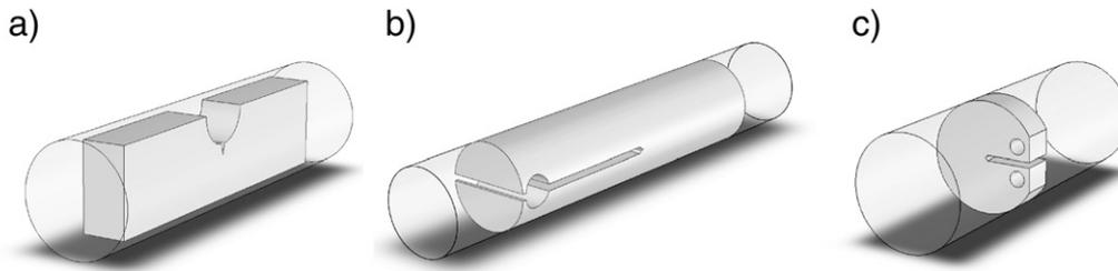
**Fig. 1.** Different specimen types manufactured out of tungsten rods. 3PB-specimen with crack direction in radial direction (a). DCB-specimen with crack direction in rolling direction (b). CT-specimen with crack direction in radial direction (c).
