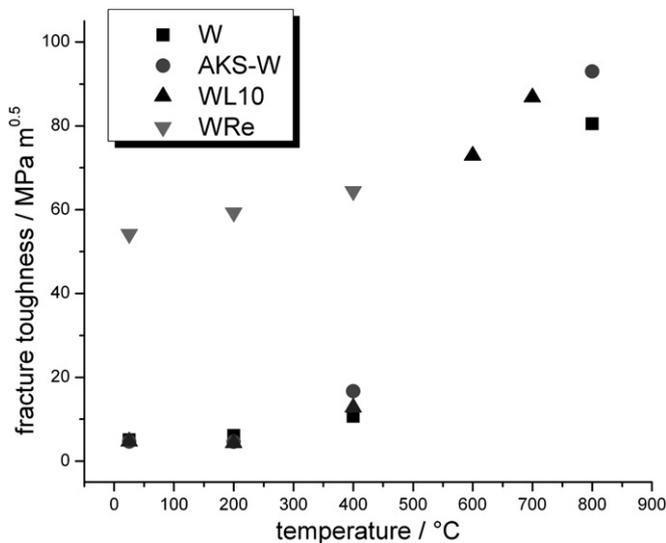
**Fig. 3.** Fracture toughness  $K_Q$  of W, AKS-W, WL10 (sintered) and WRe26 (rolled and stress relieved) as a function of temperature *T*. All values above 400 °C have been calculated from their  $COD_C$  values using Eq. (1).
