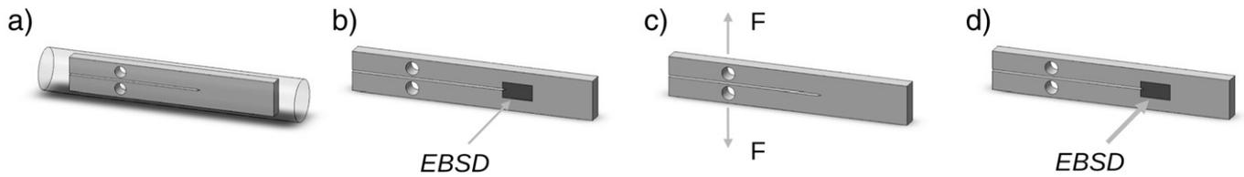
**Fig. 2.** Experimental setup to investigate the local variation of the fracture resistance: position of a DCB-specimen in a AKS-W rod (a). Scanning the area in front of the crack tip using EBSD (b). Apply a tensile load on the specimen (c). Scanning the previously scanned area again (d).
