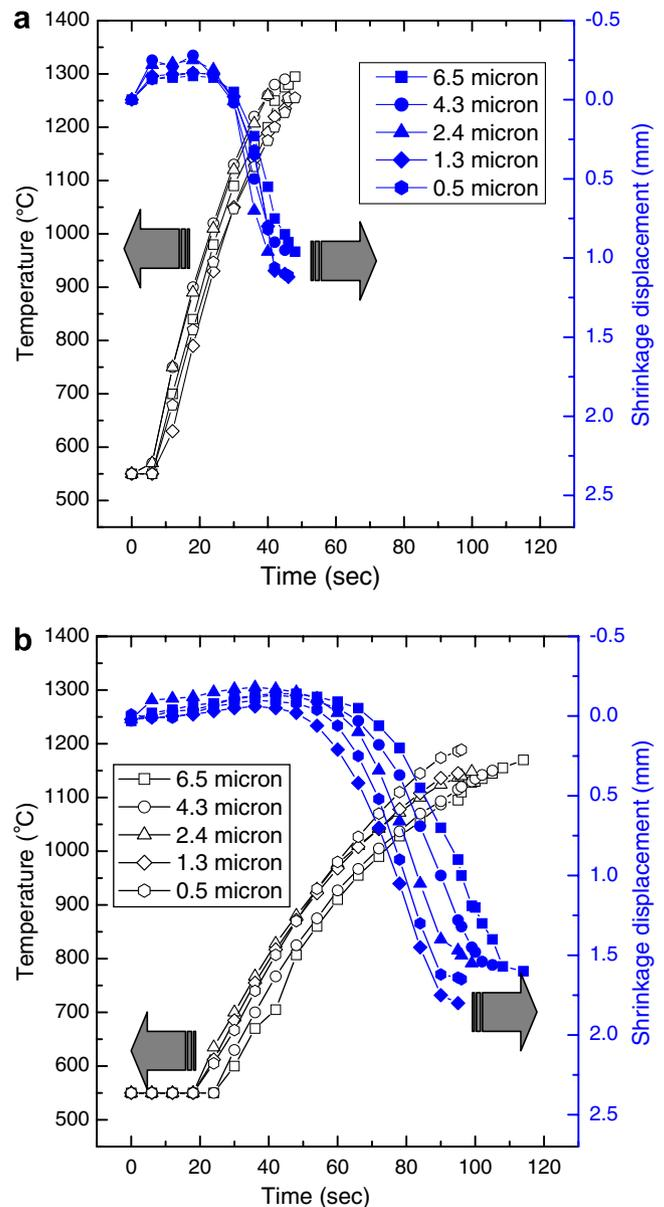
Fig. 1. Variations of temperature and shrinkage displacement with heating time for various initial particle sizes during the sintering of WC–Co hard materials (a) HFIHS and (b) PCAS.
