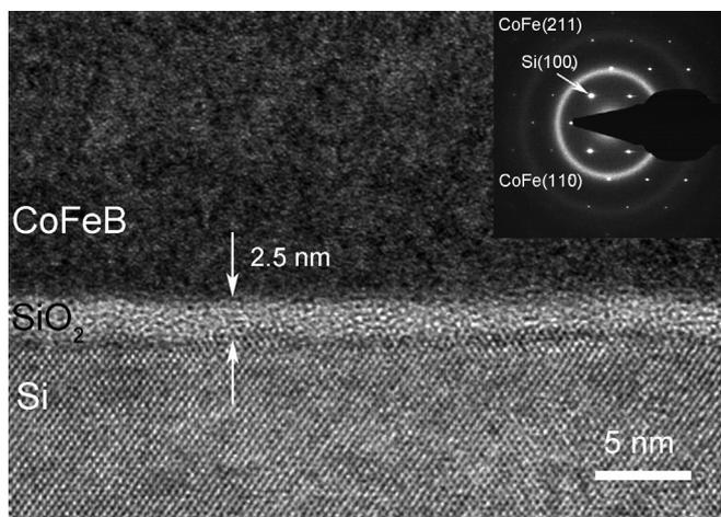
**Fig. 1.** High-resolution cross-section TEM image of  $\text{Co}_{40}\text{Fe}_{40}\text{B}_{20}$  film on  $\text{Si}(100)$  substrate, the inset is the selected-area electron diffraction patterns.
