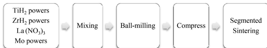
Fig. 1. La-TZM alloy sintered material preparation process flow.
