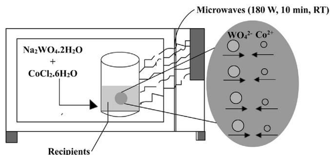
Schematic illustration of synthesis of cobalt doped  $\text{WO}_3 \cdot \text{H}_2\text{O}$  in microwave atmosphere.
