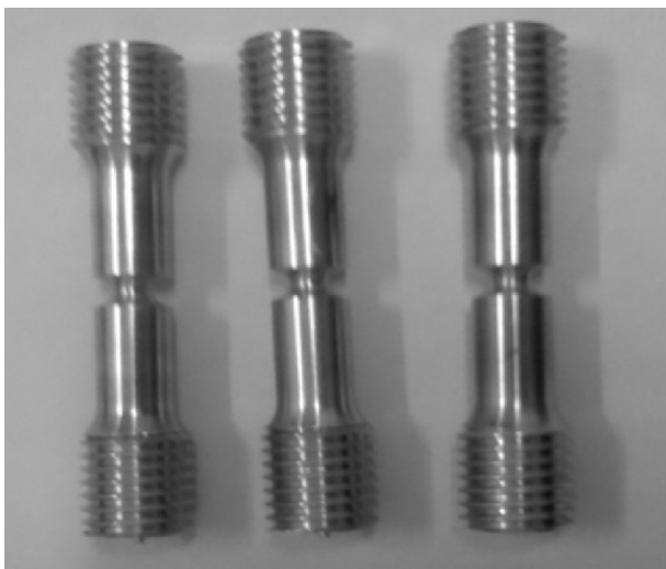
Fig. 1. Photo of the notched tensile specimen of near- \alpha titanium alloy.
