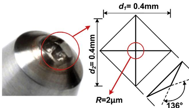
Fig. 1. Specific dimensions of the standard Vickers indenter adopted for the indentation and scratch tests.
