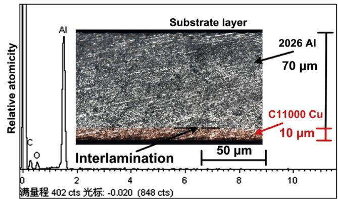
Fig. 2. Cross-section optical image of Cu/Al specimen and the energy spectrum analysis results of the substrate layer.
