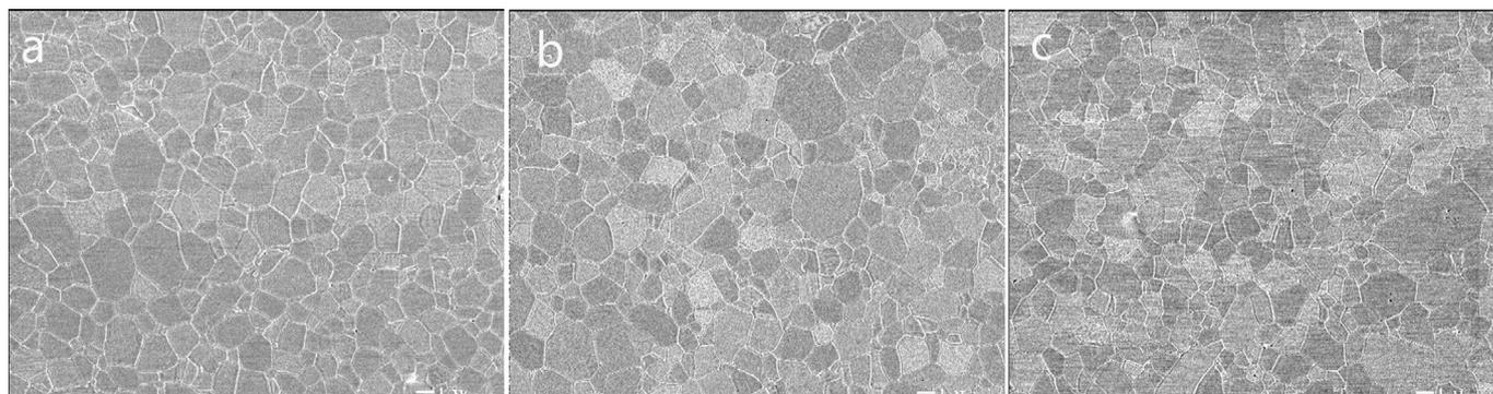
Fig. 1. Normal grain growth in La-doped alumina; Scanning electron micrographs of samples annealed at 1350 °C for (a) 8 h, (b) 12 h, and (c) 16 h.
