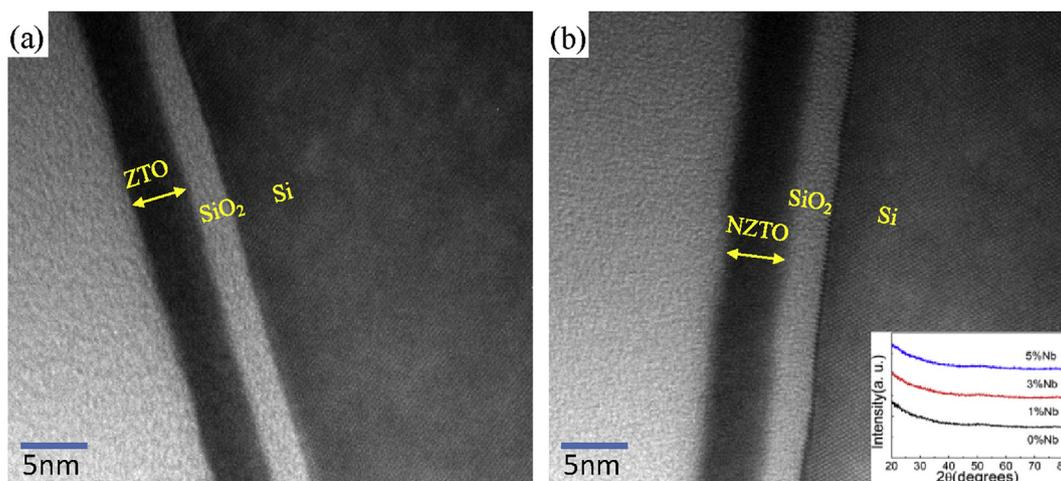
Fig. 1. Cross-sectional TEM image of solution-processed (a) ZTO film and (b) 3% Nb doped ZTO film on  $\text{SiO}_2/p^+$ -Si. Inset in Figure 1 (b) shows the GIAXRD patterns of 10-layers NZTO films with different Nb-doping concentrations.
