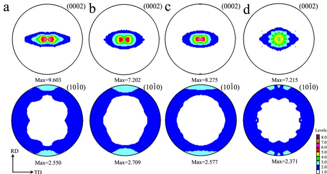
Fig. 1. Pole figures of a Mg–5.7Zn plate after hot rolling at 400 °C–39% and annealing: (a) hot-rolled (b) annealed at 400 °C for 1 h, (c) annealed at 400 °C for 3 h and (d) annealed at 450 °C for 9 h.
