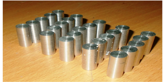
Fig. 1. Work piece made up of Aluminum 4032 composite alloy.
