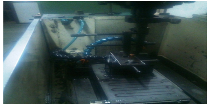
Fig. 2. EDM machine setup.
