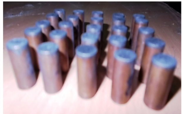
Fig. 3. Tool – copper electrode.
