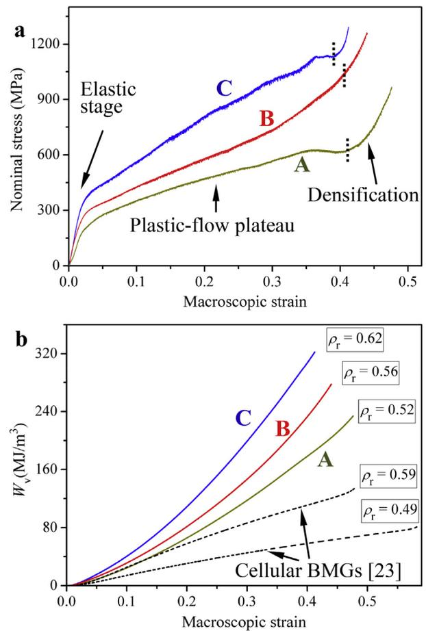
**Fig. 2.** The compressive testing results of the saw-tooth-like BMG structures (a) and the corresponding evolution of the energy absorption capacity ( $W_p$ ) of the saw-tooth-like BMG structures (b). The dash lines in (b) show the evolution of  $W_p$  of two cellular BMGs with macroscopic cellular structures [23] for comparison.
