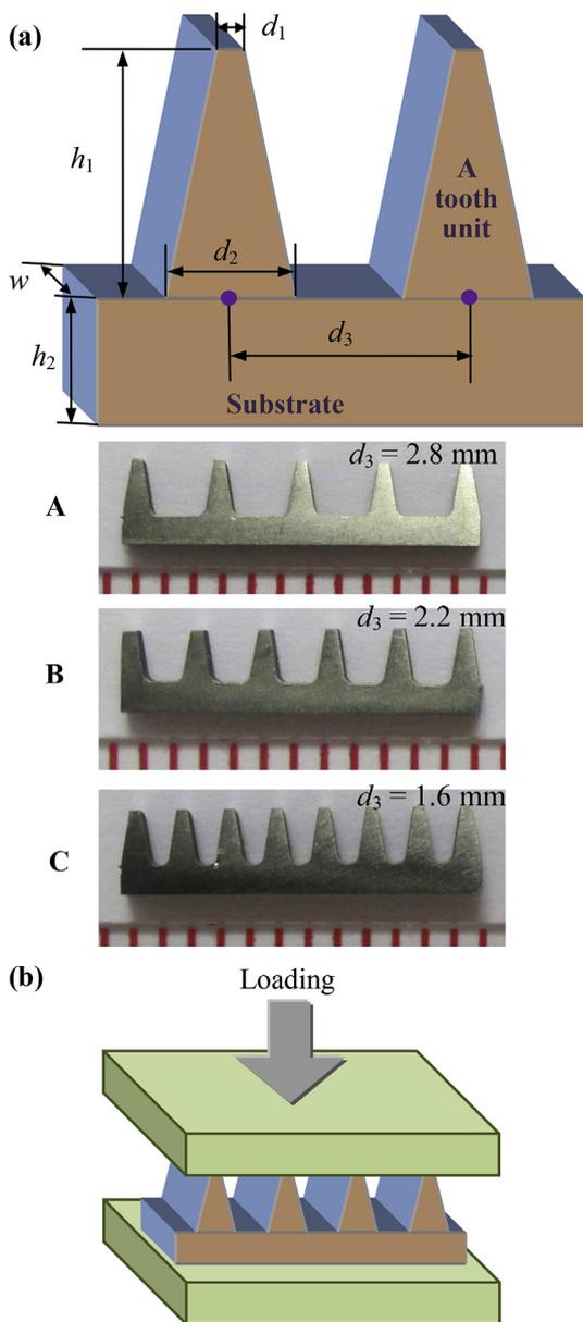
**Fig. 1.** (a) The schematic diagram of the designed saw-tooth-like BMG structures, where  $h_1 = 2$  mm,  $h_2 = 1$  mm,  $w = 2$  mm,  $d_1 = 0.33$  mm,  $d_2 = 1$  mm, and  $d_3 = 2.8$  mm, 2.2 mm and 1.6 mm respectively for specimens A, B and C, respectively. (b) The schematic diagram showing the compressive testing of the saw-tooth-like structures.
